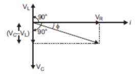
Thus,  $V_R$  and  $(V_C - V_L)$  are mutually perpendicular and the phase difference between them is 90°. As seen in the fig, we can say that, as the applied voltage across the circuit is V, the resultant of  $V_R$  and  $V_C - V_L$ ) will also be V.
