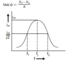
From the graph, we can see that with increase in frequency, current first increases and then decreases. At resonant frequency, current amplitude is maximum.
