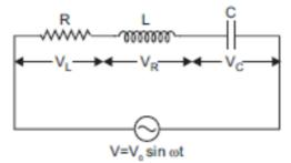
Since L, C and R are connected in series, current flowing through them is the same. The voltage across R is  $V_R$ , inductance across L is  $V_L$  and across capacitance is  $V_C$ .
